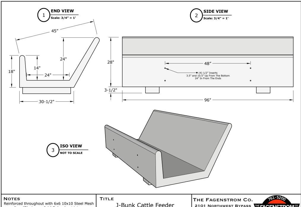
as well as (5) pieces of #4 Rebar bent into a J shape and a piece of #4 rebar running horizontally along both of the two upper edges.
